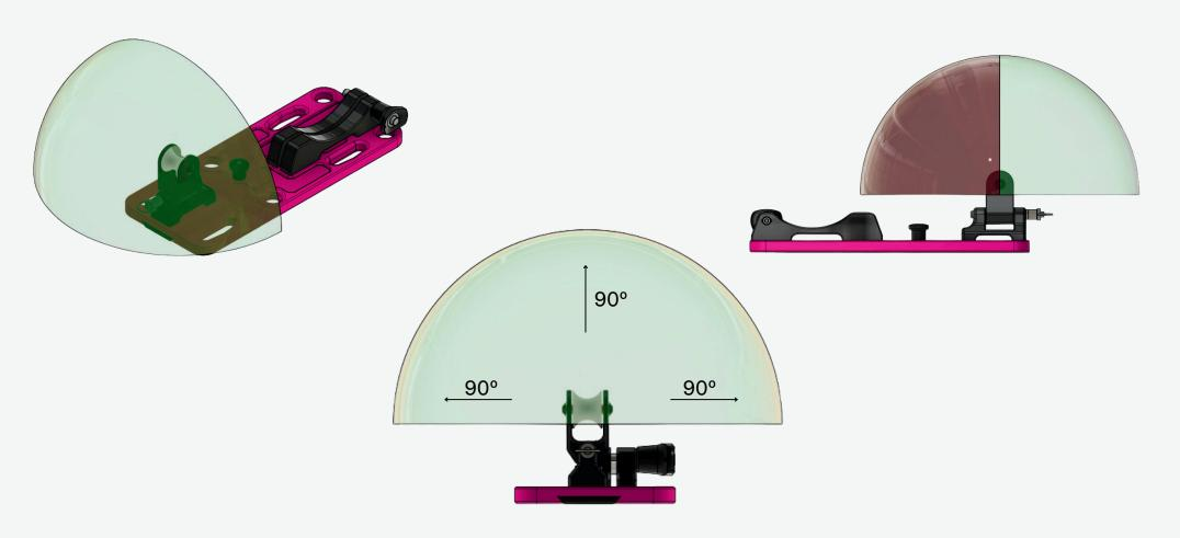
Ensure that the rope angles can't be less than 90 degrees relative to the pulley. Make sure to use the pulley.
