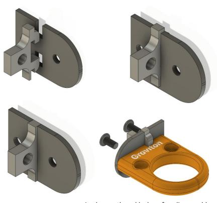
Apply new thread locker after disassembly
