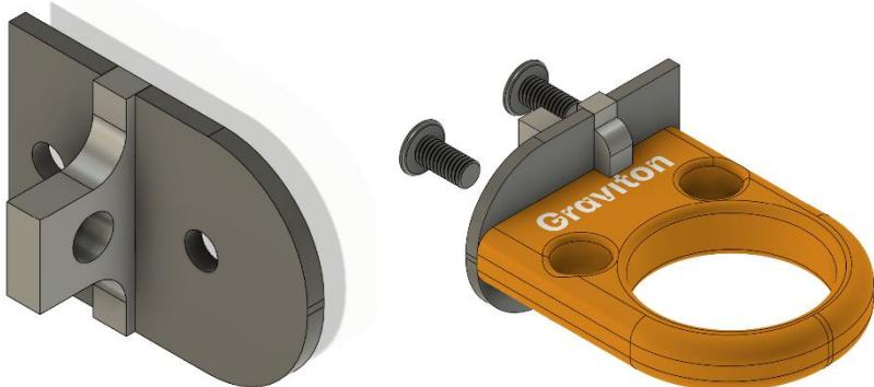
Apply new thread locker after disassembly
